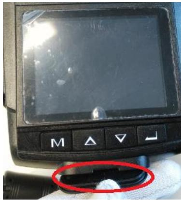
Figure 3-1 Open Cover of SIM Card Slot
