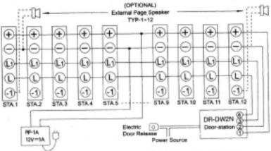
Figure-5 TP-nRC and DR-DW2N Connection Diagram
