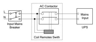
Fig.4-1 Typical external isolating device installation
