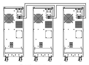
Fig.6-1 Parallel cable connect diagram
