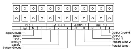
Fig.4-2 Input and output Terminal Block wiring diagram
