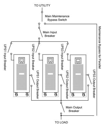
Fig.6-3 Parallel installation diagram
