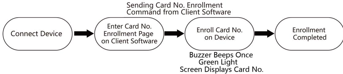
Figure 7-8 Flow Diagram of Enrolling Card
