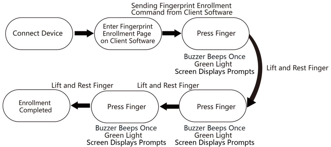
Figure 7-4 Flow Diagram of Enrolling Fingerprint
