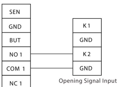
**Note:** The lock driving duration of standalone access control device needs to be set to 1s or 0s, and the door sensor needs to be set to "None".
