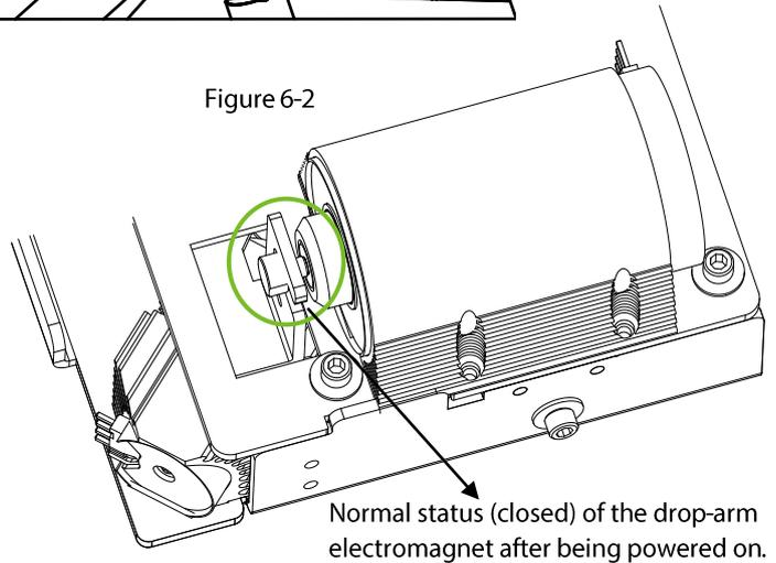
Normal status (closed) of the drop-arm electromagnet after being powered on.
