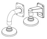
CEILING MOUNT ADAPTOR(SBP-300CM)/ HANGING MOUNT(SBP-301HM3) This adaptor is used when installing the dome camera on a concrete ceiling.
