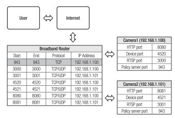
Port forwarding can be done without additional router setup if the router supports the UPnP (Universal Plug and Play) function.
