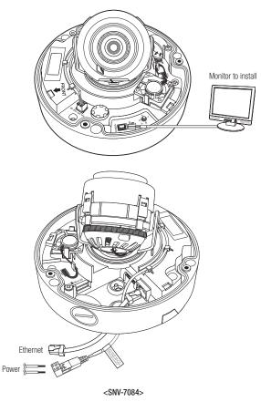
The CVBS out terminal of the product is provided for easier installation, and is not recommended for monitoring purposes.
