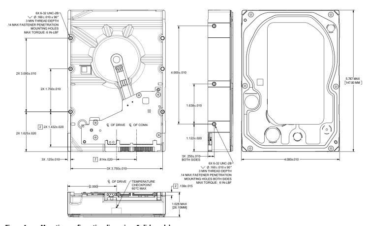
Figure 4. Mounting configuration dimensions 5-disk models
