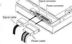
Figure 3. Attaching SATA cabling
