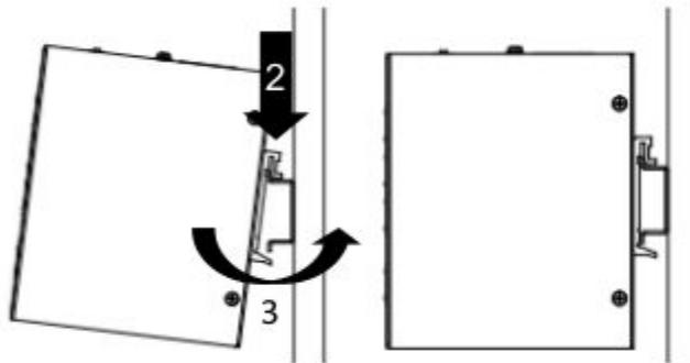
**Figure 1 — Mounting the switch on a DIN-Rail**
