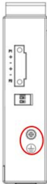
Figure 4 — The grounding screw on the switch
