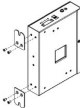
**Figure 2 — Attaching brackets to the switch**
