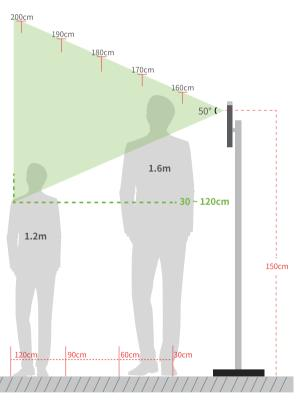
Recommended Installation Height : 150cm Temperature Measurement Distance : 30cm to 120cm
