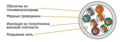
ULAN UEC-UU004-5E-PVC-GY U/UTP SOLID ETHERNET LAN CABLE 4P CATEGORY 5E PVC ( Hr(B) )
