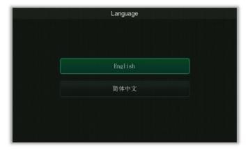
**Operation:** Press the **[OK]** button to enter the language setting, then press the **[\Delta]**/ **[\nabla]** button to switch languages. Press the **[OK]** button to confirm, the device will automatically restart, and the set language interface will be displayed after completion.
