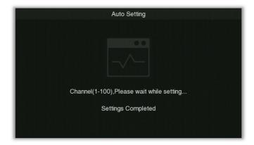
**Operation:** Press the **[OK]** button to enter the auto setting interface and the device will execute the automatic setting. When it prompts "Settings Completed", it will complete the automatic setting of the frequency band and jump to the main menu.
