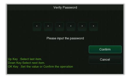
**Operation:** Press the **[OK]** button to enter the verification password input interface, then press the **[OK]** button to set the value, press the **[▲]/[▼]** button to switch, select **"Confirm"** and then press the **[OK]** button to save and exit.
