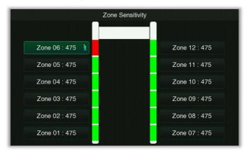
When the partition is selected for setting, the indicator light of the corresponding partition on the walk through metal detector will light up. The greater the regional sensitivity threshold, the higher the sensitivity, the effective value is 1-500, and the default value is 460.
