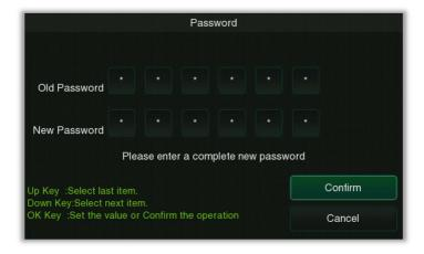
**Operation:** Press the **[OK]** button to enter the password setting interface, then press the  $[\Delta]/[V]$  button to select. Press **[OK]** button to set the value, after inputting the old password and new password, select "Confirm" and press **[OK]** button to save and exit.
