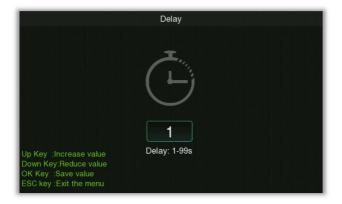
Used to set the length of time for the alarm to ring, the effective value is 1 to 99 seconds, the default value is 1 second.
