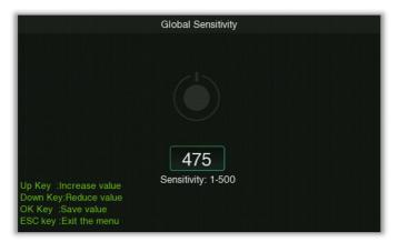
The larger the global sensitivity threshold the higher the sensitivity, and the effective value is 1 to 500, the default value is 460.
