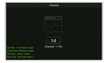
**Operation:** Press the **[OK]** button to enter the manual setting interface, then press the **[\Delta]**/ **[\nabla]** button to increase or decrease the value, press **[OK]** button to save and exit to the upper menu after finishing, directly press **[\Delta]** button to exit to the upper menu without saving the current value.
