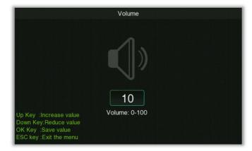
Used to set the alarm volume, the larger the value the higher the volume, valid values are 0 to 100, the default value is 80.
