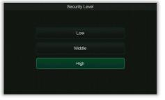
Three security levels can be set as Low, Middle and High. The higher the security level, the higher the corresponding sensitivity.
