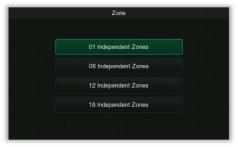
**Operation:** Press the **[OK]** button to enter the zone setting interface, then press the  $[\blacktriangle]/[\blacktriangledown]$  button to select, press **[OK]** button to save and exit.
