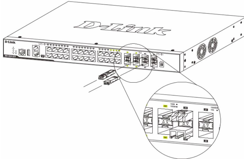
The DIS-S310R / DIS-S310T transceiver is hot pluggable. You can connect the transceiver while the system is powered on without causing any issues, and easily plug or unplug the transceiver without interrupting the network operation.
